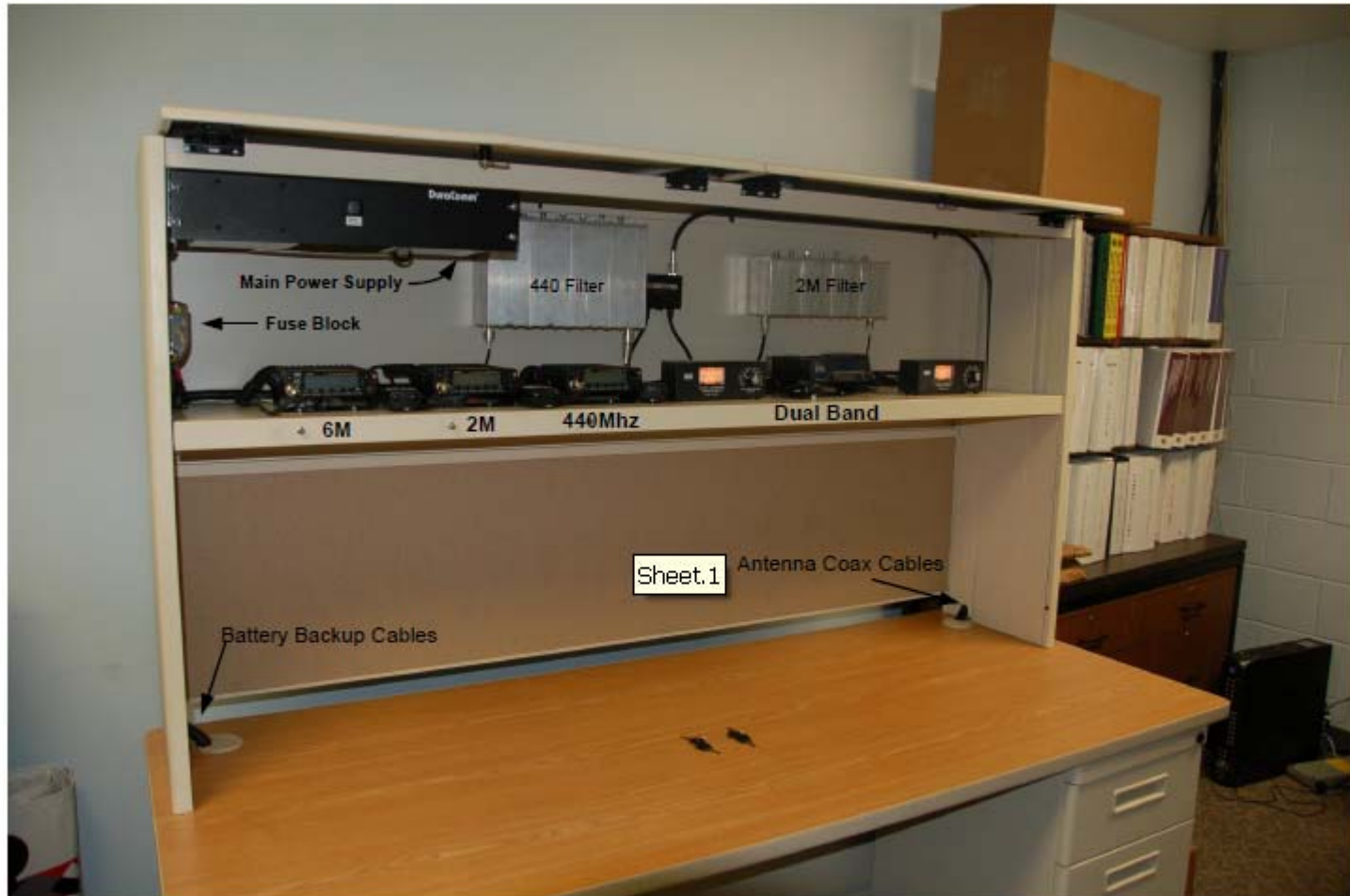
K.P.A.R.N. Radio Equipment mounted in Desk with Locking Hutch
